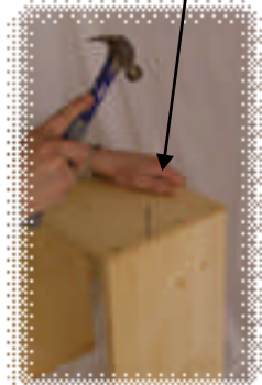
STEP 2: Nail at each end using 6d sinkers— 4 nails.
